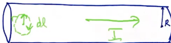
Figure 15: A current-carrying wire with an Amperian loop of radius r and clockwise direction for d\vec{l} .
